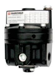
A pneumatic air volume booster reproduces a low flow control signal with a greater flow regulated output pressure. It uses an unregulated input pressure to maintain a regulated output pressure under flowing and non-flowing conditions.
