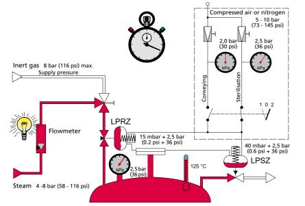
Initially the steam condenses at the cold container wall. The pressure increases slowly. The pressure and the corresponding temperature are constant at any point in the sterile zone. The steam flow rate falls to the quantity required for compensating the temperature loss through convection.
