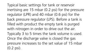
After purging the tank is filled with product. For this the product outlet valve closes and the inlet valve is opened. With increasing product level in the tank the pressure in the headspace increases until the set value of 40 mbar (0.6 psi) is reached. Nitrogen is then discharged via the back pressure regulator into the gas processing unit or atmosphere.
