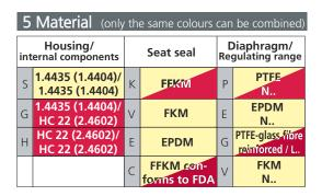
Example: Housing/internal components with material code "G" or "H" (red) are only combined with seat of type "K" or "C" and with diaphragm type "P" or "G".
